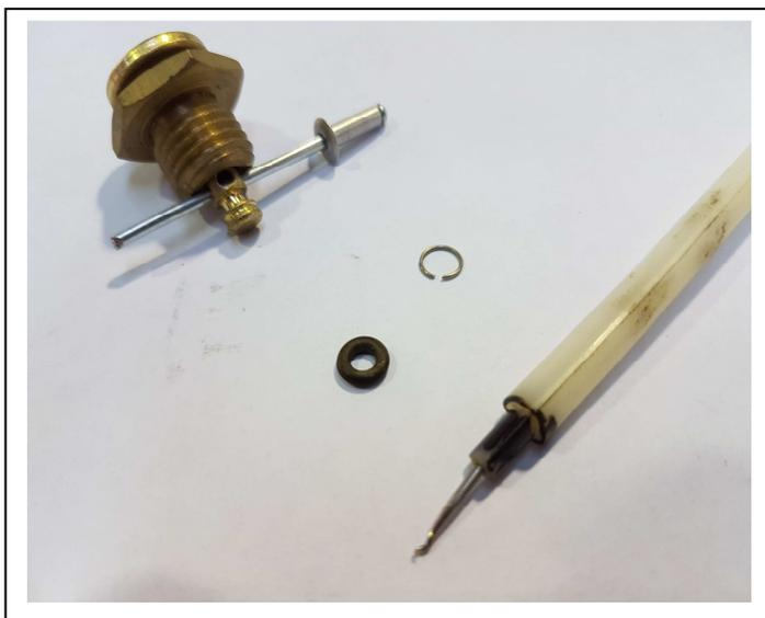
Compress spring in body and place shear part of 1/8" rivet or similar in cross holes to hold spring compressed. SEE PHOTO.
