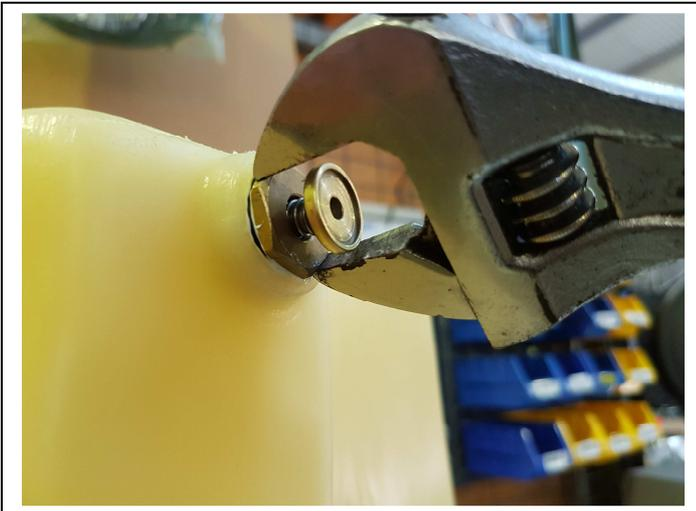
Use adjustable wrench or similar, to remove the draincock assembly.
