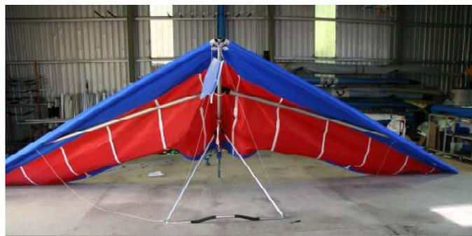
Figure 4 Section 4. Spreading the leading edges
