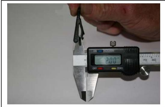
**Figure 15 Batten End Fitting Dimension Check**
