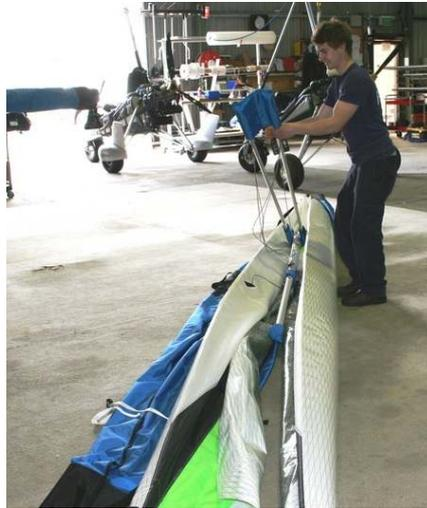
Figure 1 Section 5. Unzip wing bag
