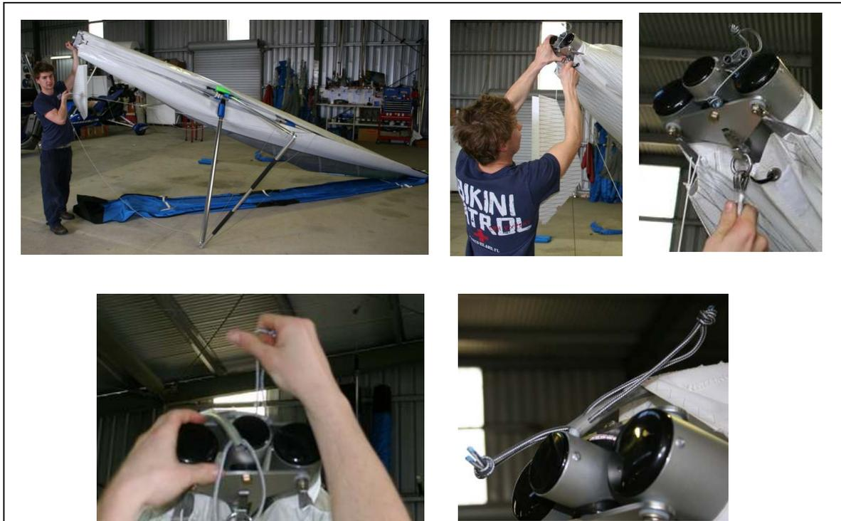
Figure 3 Section 5. Stand the wing up
