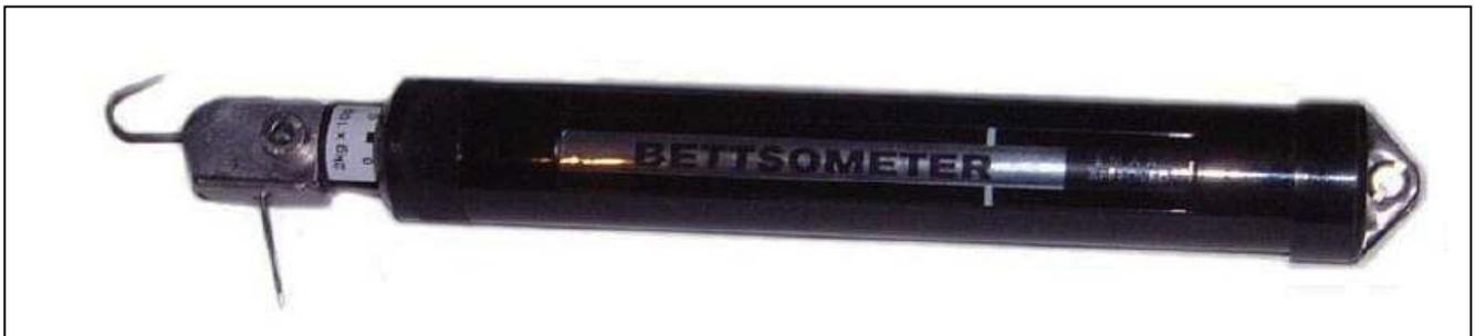
**Figure 16 Bettsometer Instrument**
