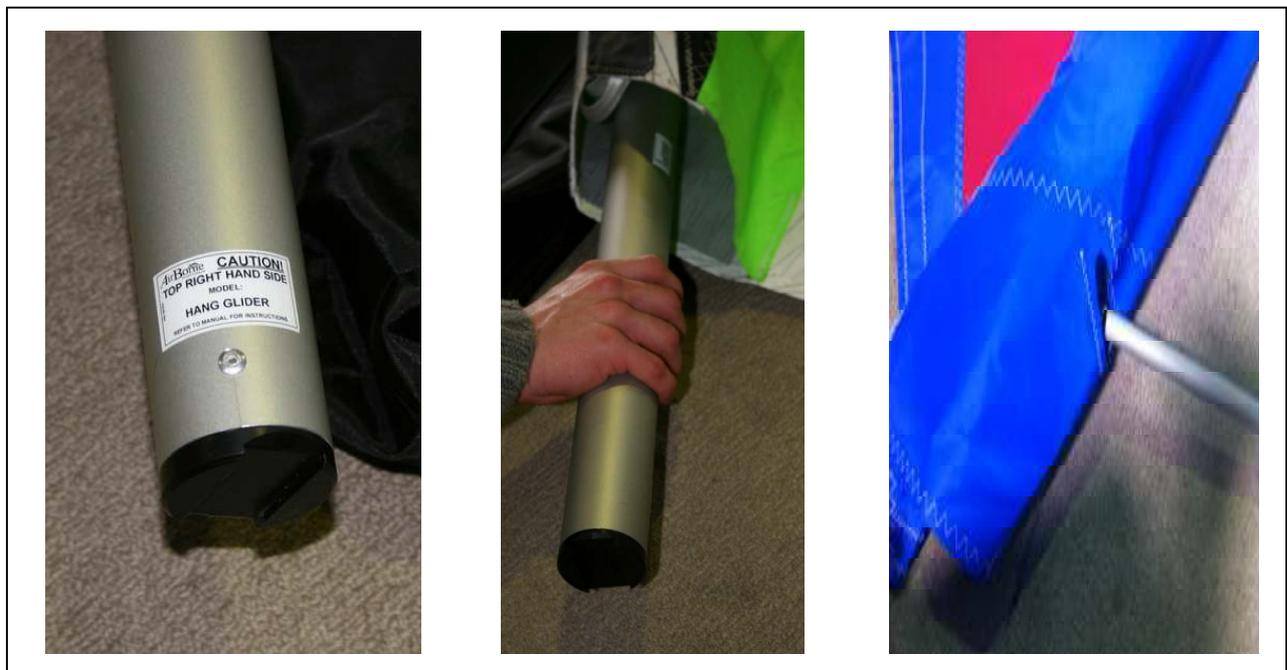
Figure 11 Insertion of Rear Leading Edges
