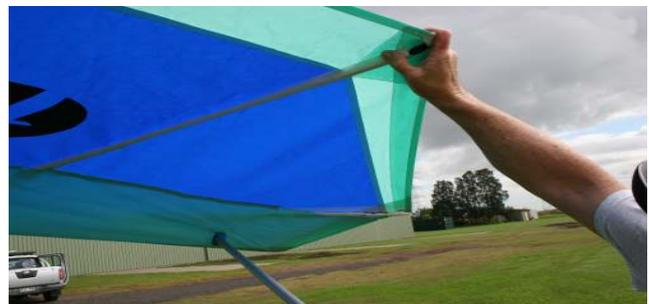
Figure 9 Section 5. Install Washout Rod
