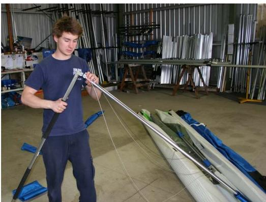
Figure 2 Section 5. Assemble control frame
