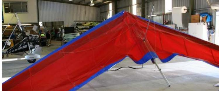
Figure 5 Section 5. Raise king post and connect reflex bridle
