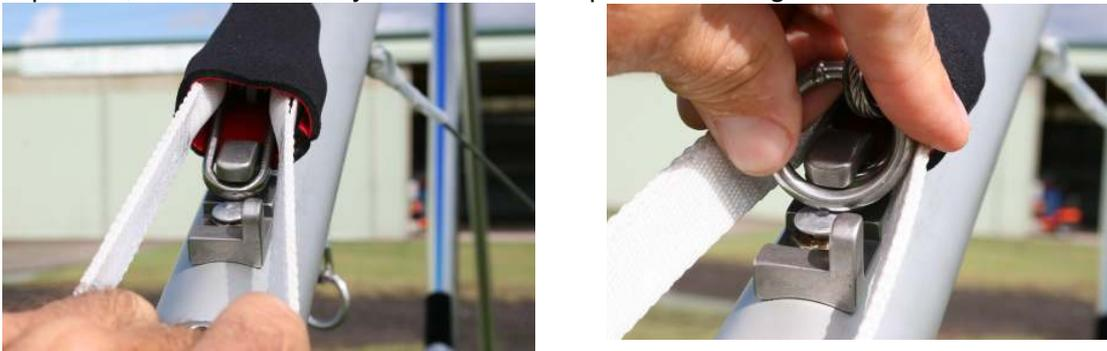
Figure 7 Section 5. Tensioning cross bar and shackle located in block
