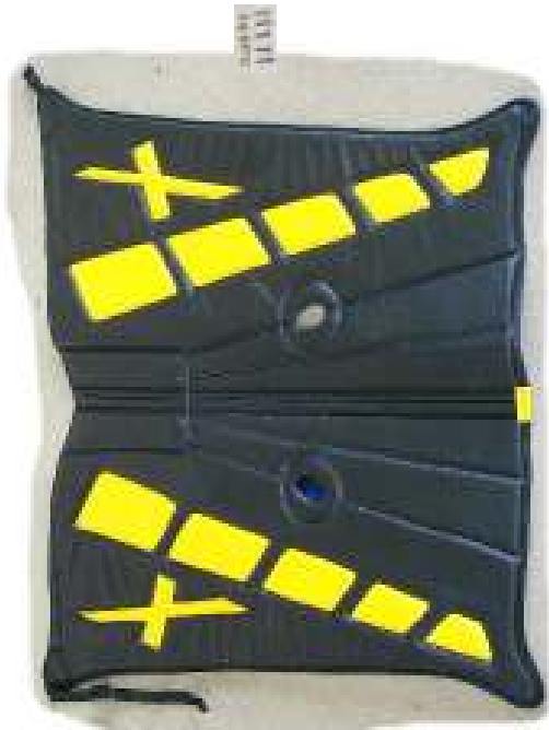
COMPLETED SOFT SIDES AND FIXING SCREWS
