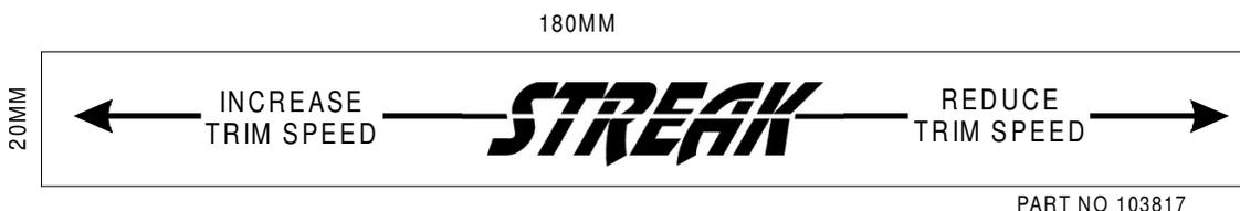
The wing trimmer operation placard is fitted to Streak wings only. It is located on the control frame starboard down tube adjacent to the trimmer knob.
