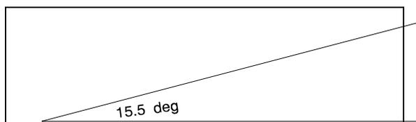
It is necessary to set the blade angle so that the space between the leading edge and the template is equal to the space between the trailing edge and the template. As you adjust each blade tighten the bolts just enough to stop the blade from rotating while you are adjusting the other blades.
