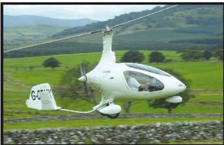
ALL flying machines with lifting surfaces MUST continually deflect air downward to counteract weight to remain in straight and level flight. Constant auto-rotation during steady straight and level flight can generally only be maintained with the rotor 'disk' tilted away from the direction of flight by something like 8 or 9 degrees.
