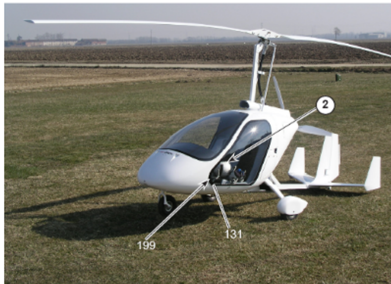
Fig. 3.5/1 Disassembly of rotor and head
