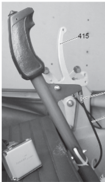
Fig. 3.2/1 Prerotation control cable adjuster
