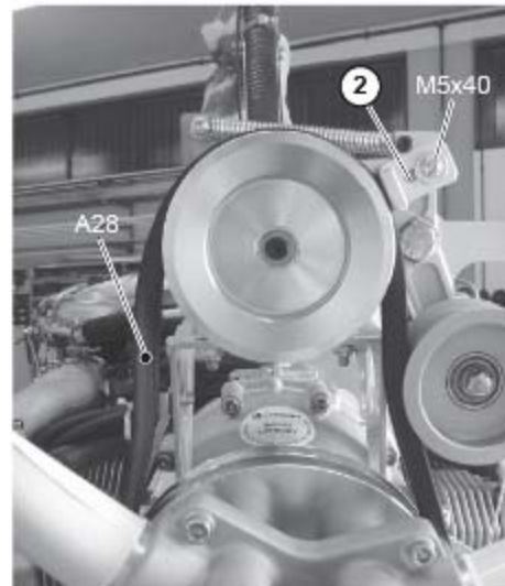
Fig. 3.2/4 Shoe (2) in contact with the belts (correct position)
